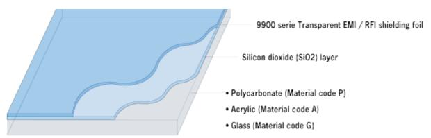
Technical drawing of the construction in layers of the 9910 series Transparent EMI shielding foil windows
