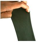
Stretch conductive fabric can be well stretched and remains electrically conductive
