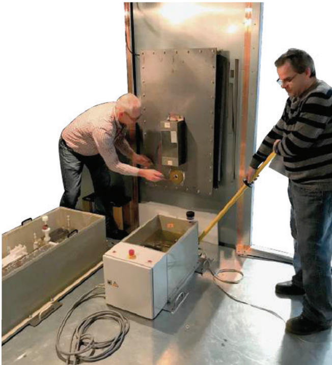
E1/E2 test conductive (N)EMP test filter
