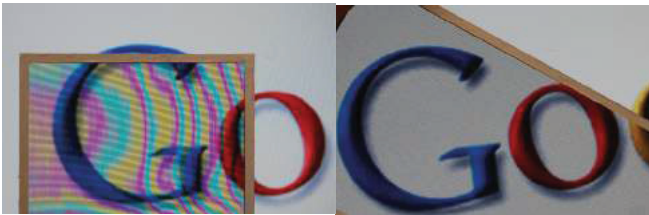
Mesh foil with moiré effect and without moiré effect
