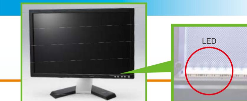
When the light comes out from encapsulant to the air gap, and comes into the light guide panel, a reflection loss occurs due to the difference of refractive index of the air and the parts, which leads to decrease of luminance. Applying **OPT $\alpha$ GEL** prevents the reflection loss, and improves the luminance.
